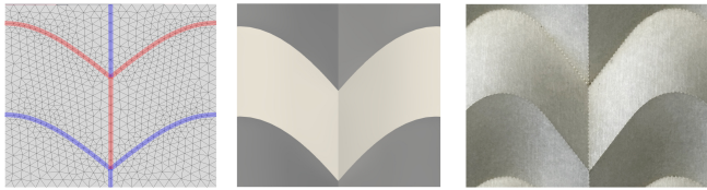
Fig. 2. Unit-cell model. Left: Periodic triangle mesh conforming to crease pattern with mountain-valley assignments indicated in red and blue, respectively. Middle: simulation result for folded configuration. Right: corresponding physical prototype with pre-scored creases.
