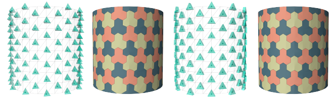
Fig. 8. Comparison of a fixed-orientation tetrahedral metric (left) with a surface-aligned triangular extruded metric (right). For each, a visualization of site locations and metric polyhedra is shown along with the resulting Voronoi diagram. The extruded metric enables consistent shape of Voronoi cells around the cylinder, where cells in the fixed metric example become distorted due to misalignment.
