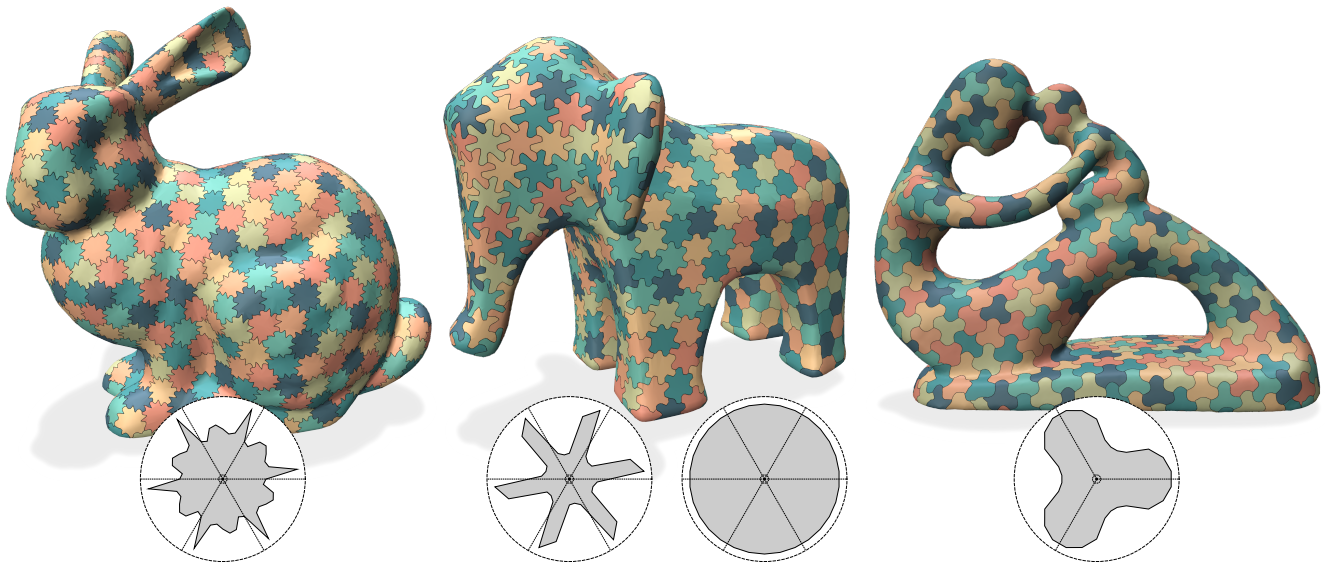
Fig. 1. Our closed-form construction enables restricted star-shaped distance Voronoi diagrams on 3D surfaces. Left : metric with six-fold rotational symmetry. Middle : interpolation between star-shaped and Euclidean distance metric. Right : metric with threefold rotational symmetry. Diagrams under each example show the metric polygons defining each star-shaped distance function.
